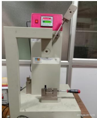
Figure 4 Composite coupon placed in impact testing machine for the conduction of impact test
