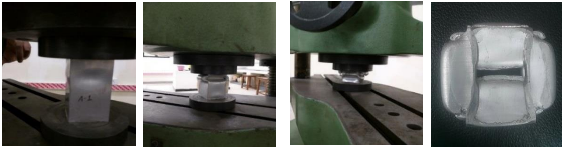
Fig. 4. Axial Crushing of Empty Tube at different stages of loading
