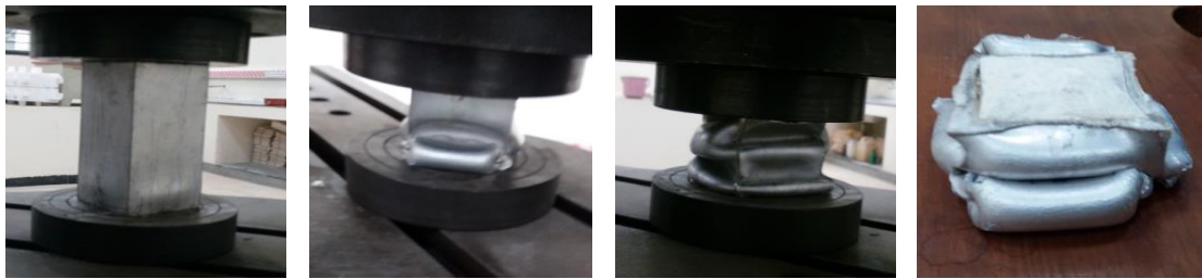
Fig. 5 Axial Crushing of Tube filled with polyurethane foam at different stages of loading
