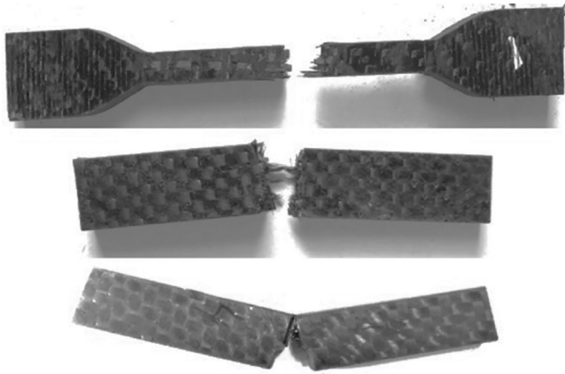
Fig. 7. Fractured specimens after testing.
