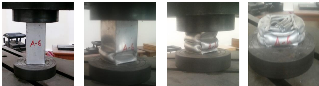
Fig. 7 Crushing of Tube filled with Pyramid Structure
